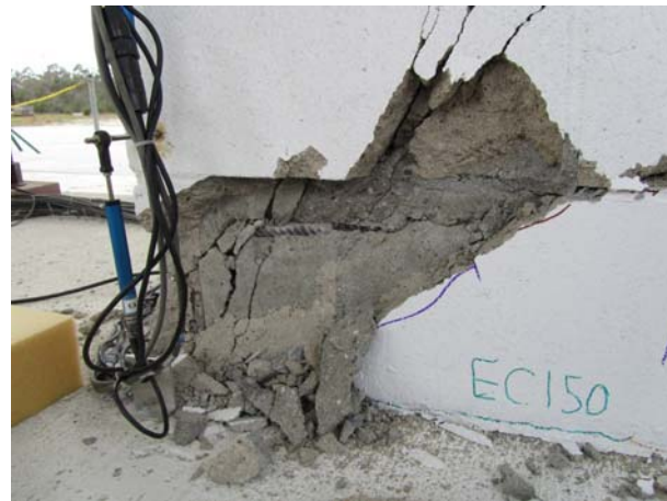
Figure 3-25 Toe at base of Wall 3 after second run of 150% Chi Chi
