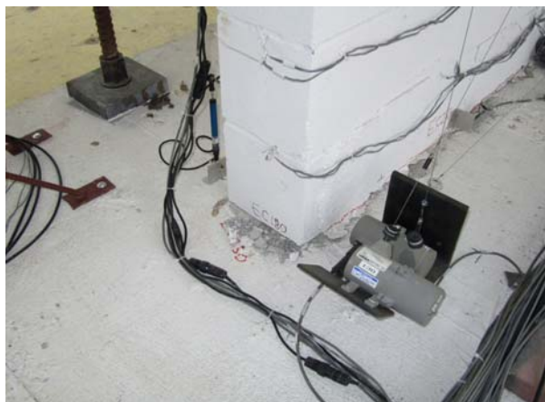
Figure 3-14 Base of Wall 2 after 100% Chi Chi
