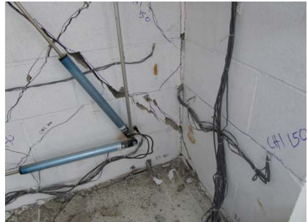
Figure 3-23 Base of Wall 1 after second run of 150% Chi Chi
