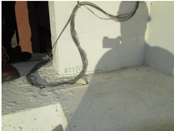
Figure 3-4 Flexural crack at base of Wall 1 flange after 150% El Centro 1979
