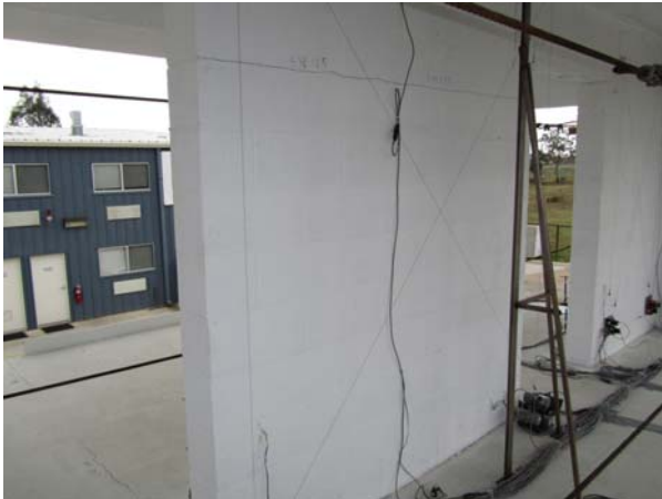
Figure 3-12 Wall 2, second story after 100% Chi Chi
