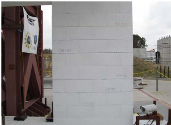
Figure 3-18 East out-of-plane wall after first run of 150% Chi Chi
