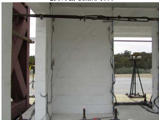
Figure 3-8 Shear cracking of Wall 1 after 100% Chi Chi
