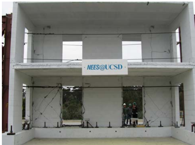
Figure 3-19 Specimen after second run of 150% Chi Chi
