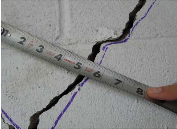
Figure 3-26 Shear crack on ground story of Wall 1 after second run of 150% Chi Chi
