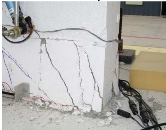
Figure 3-24 Toe at base of Wall 3 after second run of 150% Chi Chi
