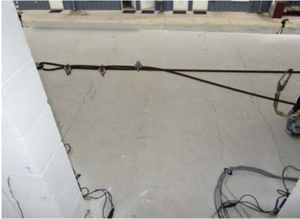
Figure 3-10 Cracks on 2 nd level slab after 100% Chi Chi
