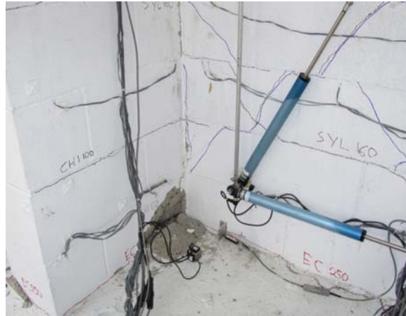
Figure 3-13 Base of Wall 3 after 100% Chi Chi
