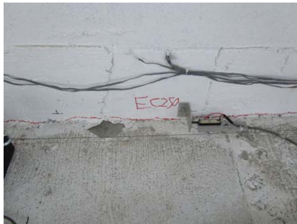
Figure 3-7 Evidence of minor base sliding of Wall 2 after 250% El Centro 1979
