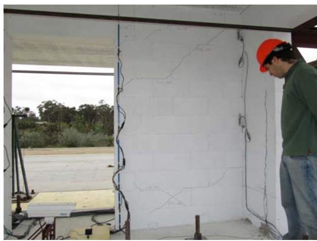
Figure 3-9 Shear cracking of Wall 3 after 100% Chi Chi
