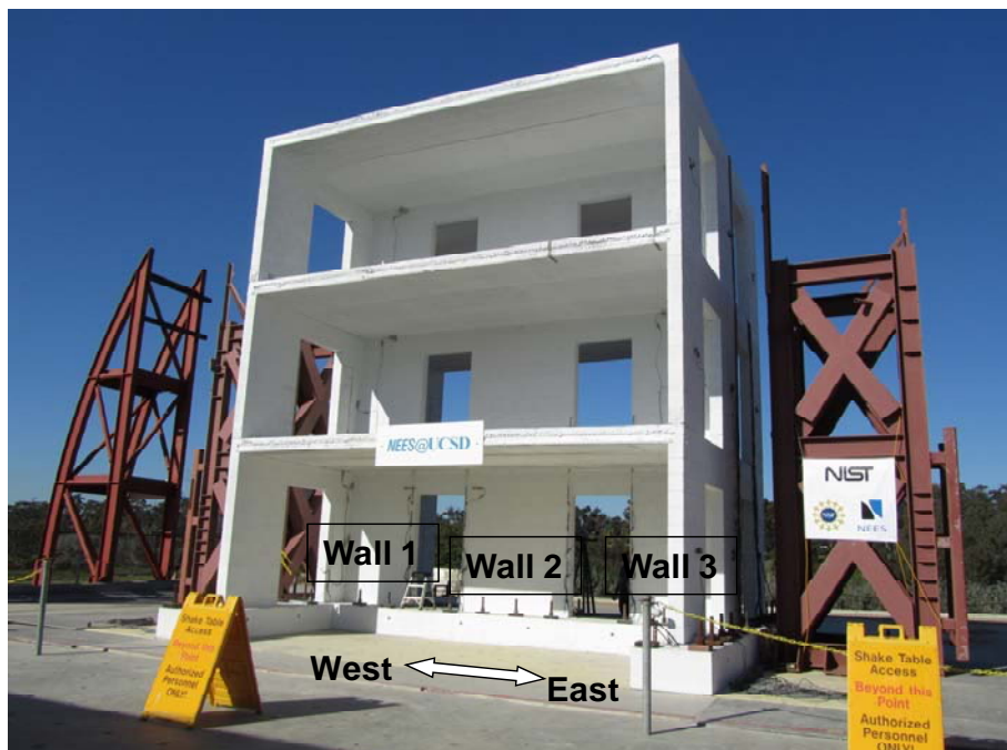
Figure 1-2 3-story, full-scale masonry specimen as constructed on UCSD shake-table
