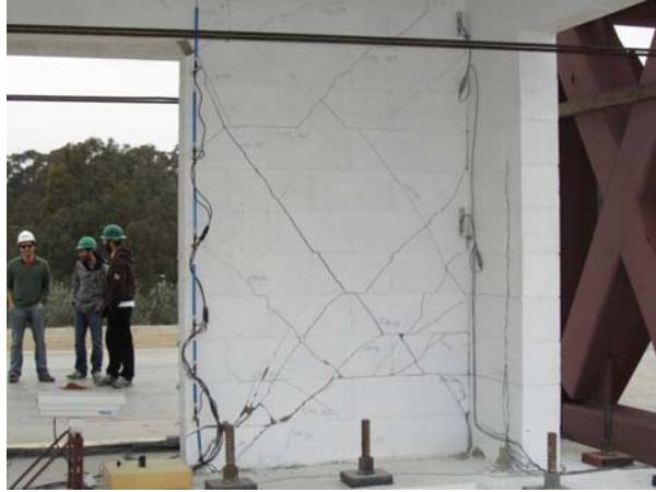
Figure 3-21 Base of Wall 3 after second run of 150% Chi Chi
