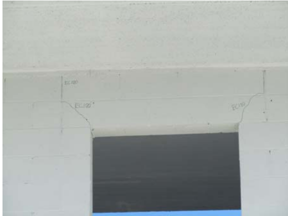
Figure 3-2 Lintel cracks after 120% El Centro 1979
