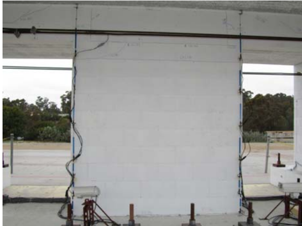
Figure 3-16 Wall 2 after first run of 150% Chi Chi
