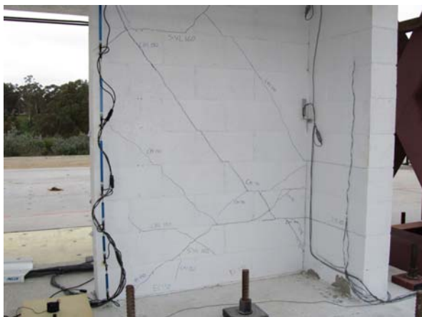
Figure 3-15 Wall 3 after first run of 150% Chi Chi
