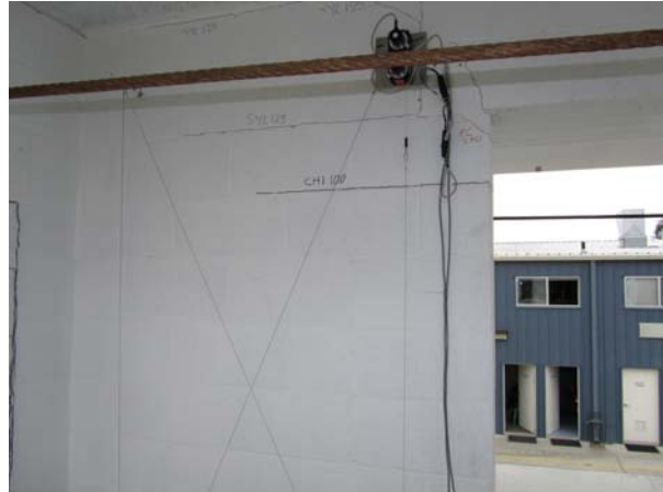
Figure 3-11 Wall 3, second story after 100% Chi Chi
