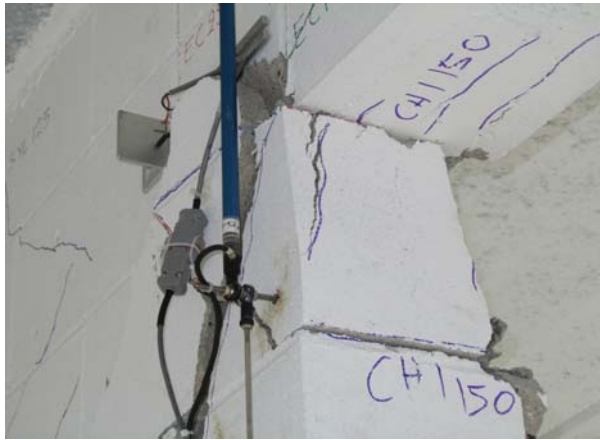
Figure 3-22 Corner of first-story lintel beam after second run of 150% Chi Chi
