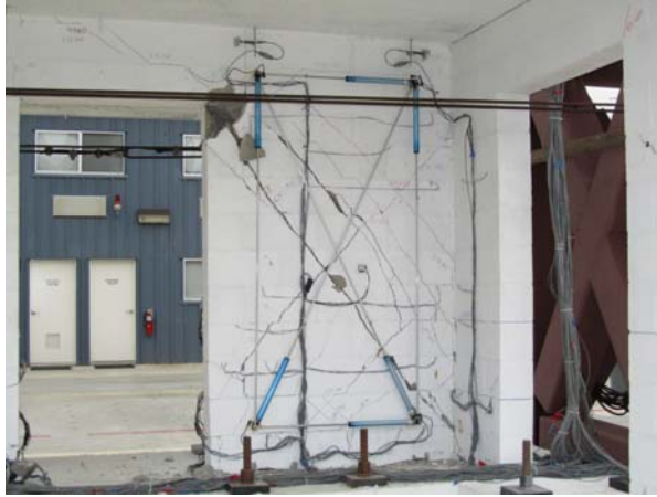
Figure 3-20 Base of Wall 1 after second run of 150% Chi Chi
