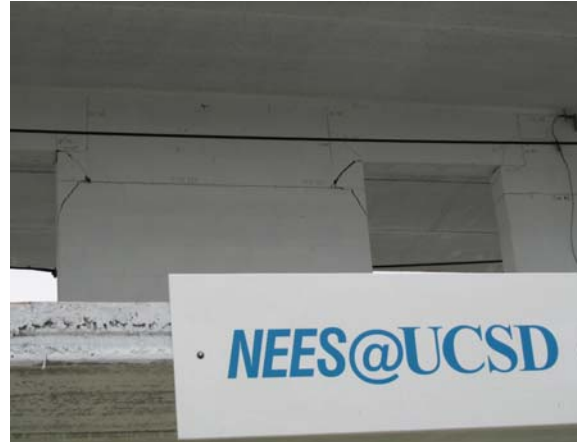
Figure 3-27 Wall 2 at second story after second run of 150% Chi Chi
