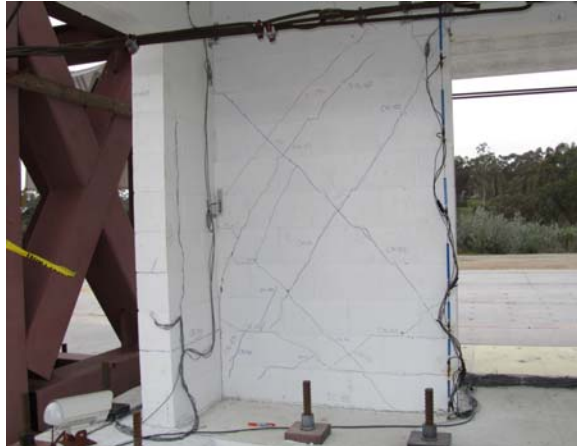
Figure 3-17 Wall 1 after first run of 150% Chi Chi
