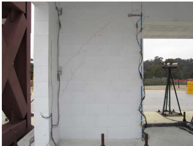
Figure 3-6 Shear cracks on web of Wall 1 after 250% El Centro 1979
