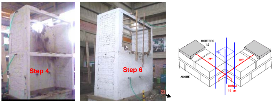
Figure 6. Shaking table test and horizontal reinforcement proposed
