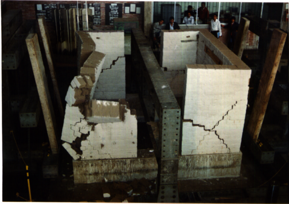
Fig. 11 Shaking table test on unreinforced wall (left) and wall with type 1 reinforcement (right)
