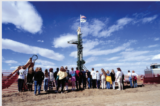
FIGURE 5.3 Drilling rig collecting the 660-m Kiowa core from the Denver Basin project, which enabled the “Castle Rock Rainforest” to be dated at 64 Ma based on recovery of 35 ash layers spanning a 4-million-year section (Raynolds and Johnson, 2002).
