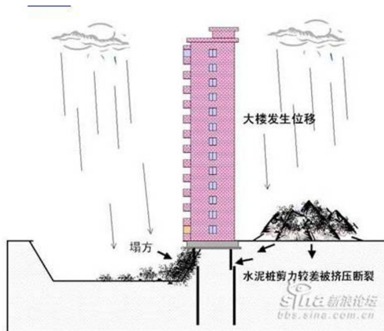
The building began to shift and the concrete pilings were snapped
