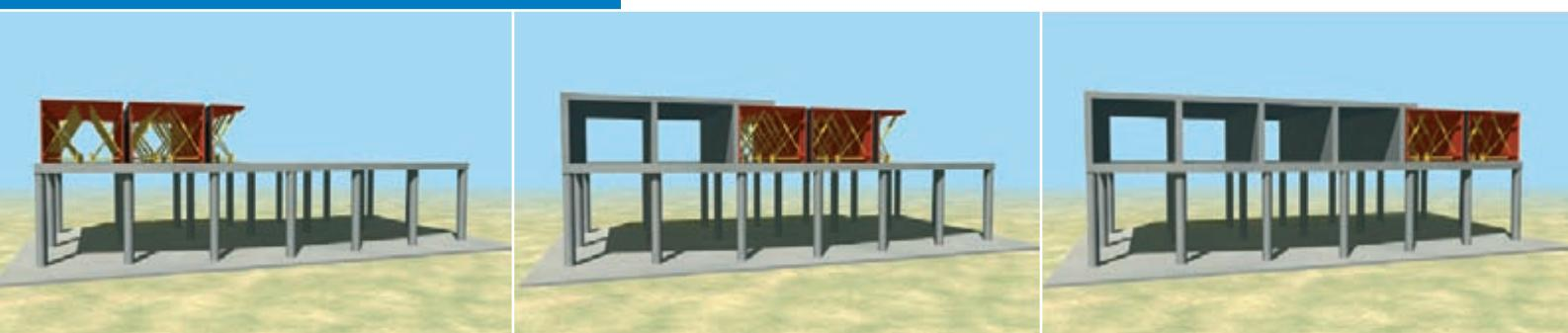
The high levels of dimensional accuracy achieved with tunnel form and the superior load distribution result in a strong, solid monolithic structure suitable for a multitude of uses. The ability to create clear spans up to 11 m wide provides the opportunity to use non load-bearing internal partitions that can be moved to provide alternative layouts.
