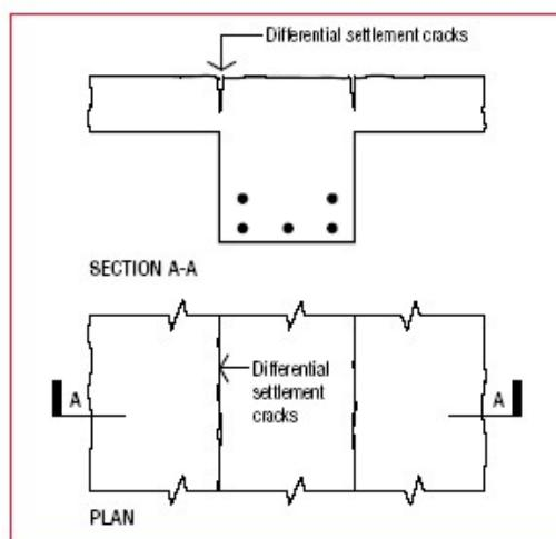
**Figure 2** Differential settlement cracking
