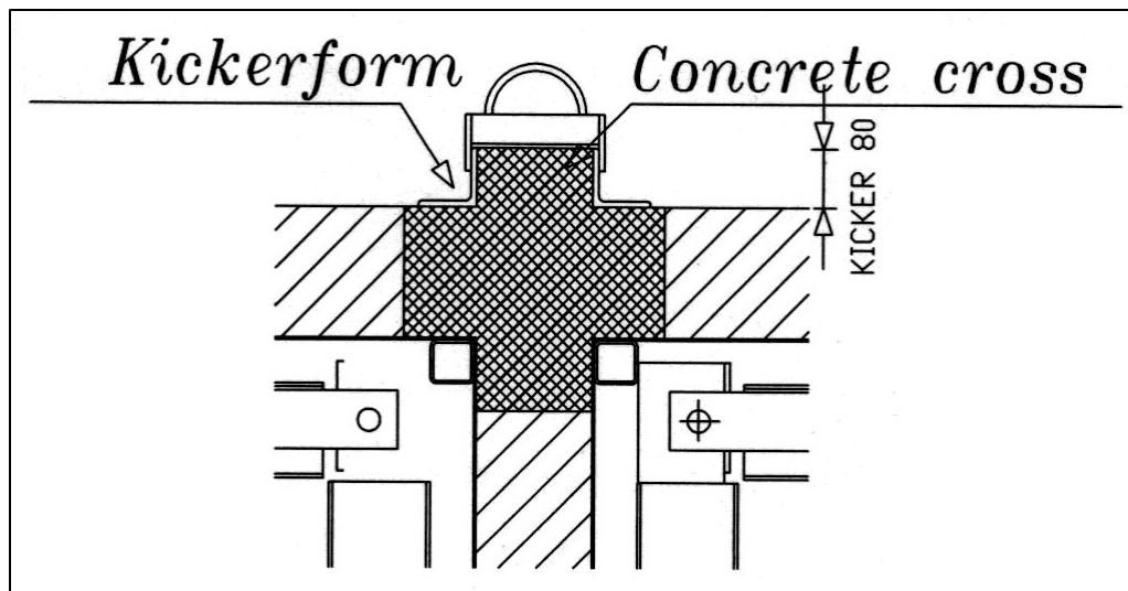
If there is to be another level added, the starter walls are formed as shown above using the steel hangers plus either precast blocks for inner walls or the angle and spacer for the
