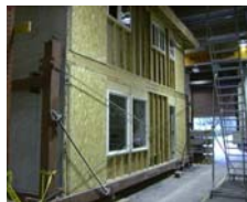
House 2: Test 09 Engineered OSB + GWB
